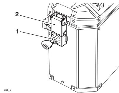
1. Lock barrel - unlock position
