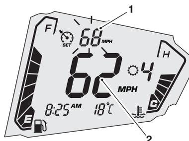
1. Cruise control set speed (flashing)
