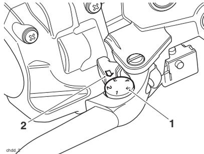
1. Adjuster wheel, brake lever shown
