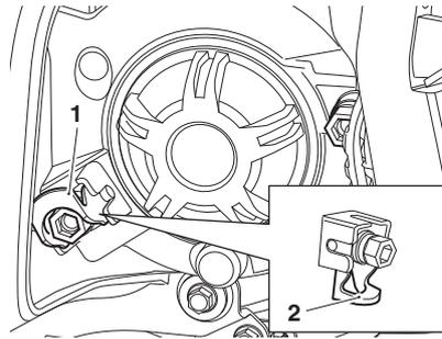
1. Headlight adjuster lever (unloaded position)
