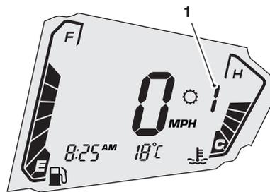
1. Gear position display (first gear shown)
