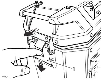
1. Pannier lid hinge quick release mechanism
